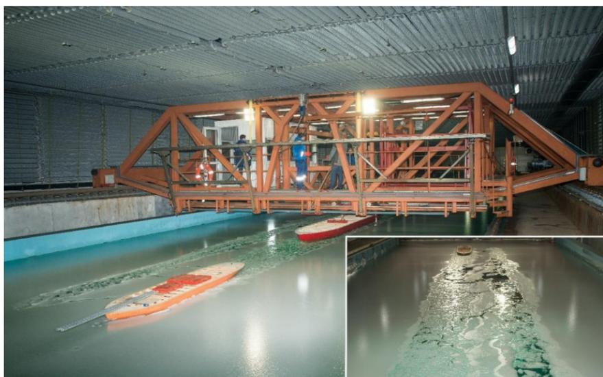
Fig. 3 – Simulation of heavy-tonnage tanker pilotage by two icebreakers (bottom right – channel formed by two icebreakers)
