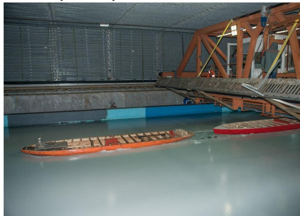
Fig. 5. Model studies: movement of a heavy-tonnage vessel model along the channel laid by an icebreaker model.
