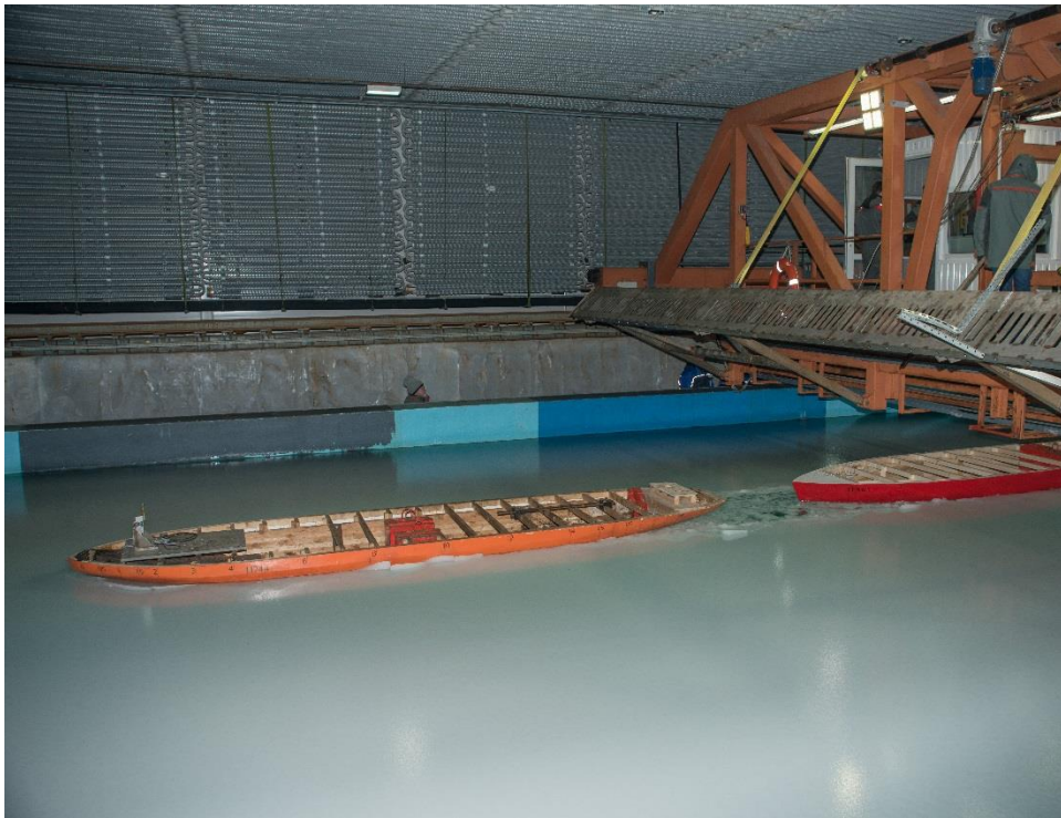
Fig. 5. Model studies: movement of a heavy-tonnage vessel model along the channel laid by an icebreaker model.
