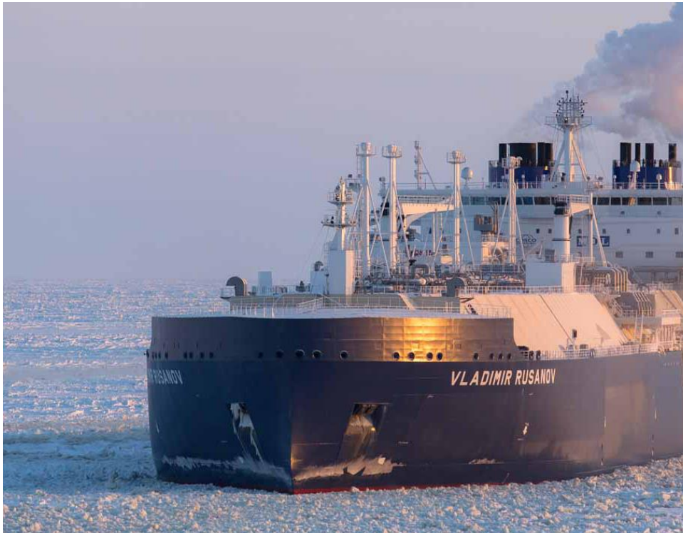
Fig. 2. "Vladimir Rusanov", the Yamal Max type heavy-tonnage vessel for LNG transportation (photo by D.V. Labuzov, dmitry-v-ch-l.livejournal.com)
