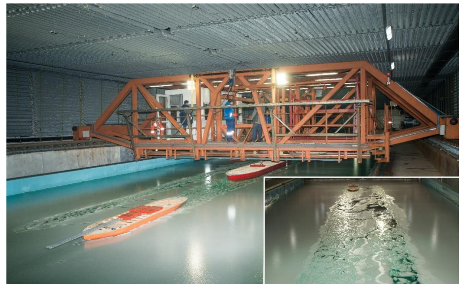
Fig. 3 – Simulation of heavy-tonnage tanker pilotage by two icebreakers (bottom right – channel formed by two icebreakers)
