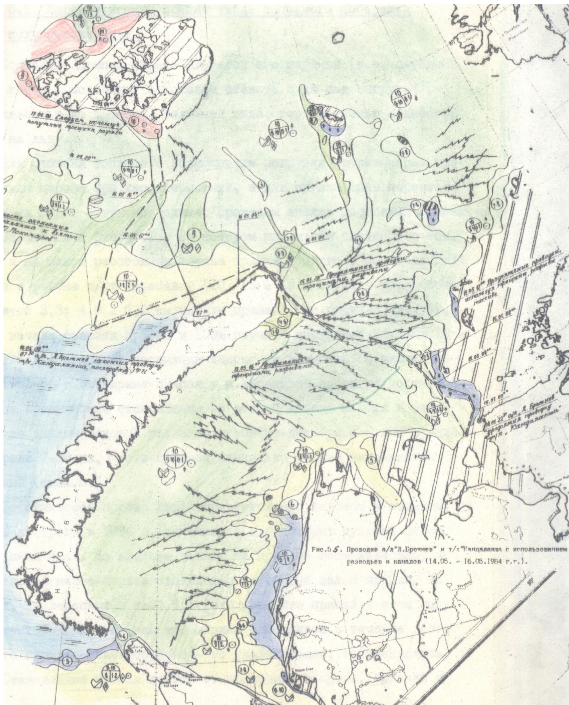
Fig. 3. Sea ice reconnaissance chart for the Kara Sea for May 14-16, 1984. Ice chart is based on visual and instrumental airborne observations accompanied by satellite data [13] (Source: the AARI archives).
