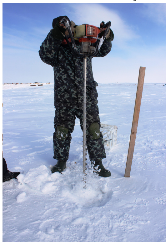
Figure 1 – Drilling of sea ice for further ice thickness measurements (research station 'Ice base Cape Baranov', Severnaya Zemlya Archipelago, May 2014). Photo: V.Borodkin.
